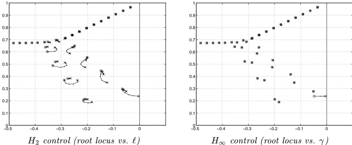
FIGURE 4. Movement of closed-loop eigenvalues versus control parameters  $\ell$  and  $\gamma$  for  $H_2$  (optimal) and  $H_\infty$  (robust) controllers applied to the Orr-Sommerfeld equation for  $Re = 10,000$ ,  $k_x = 1$ ,  $k_z = 0$  using blowing/suction as the control variable.
