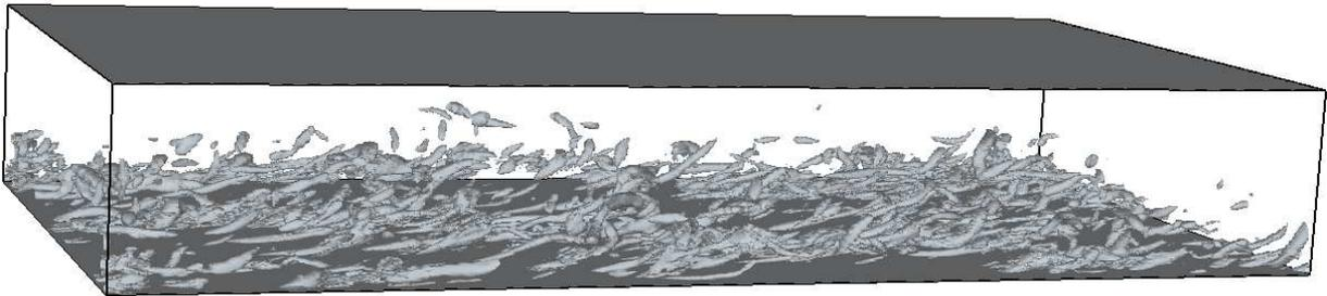
FIGURE 1. Coherent structures of a turbulent flow at  $Re_\tau = 180$ .
