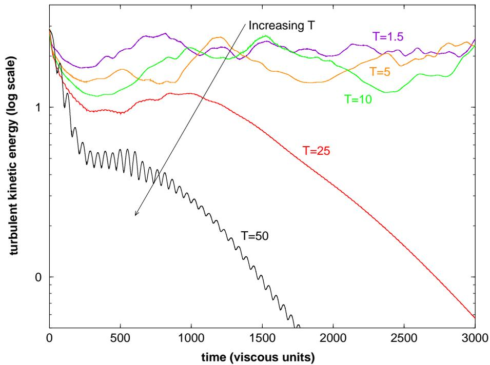
FIGURE 3. Time Evolution of the turbulent kinetic energy for different values of  $\tau$  (denoted  $T$  in the figure).
