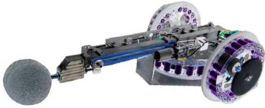
Fig. 2. Reconfigurable wheeled rover with hopping capabilities.
