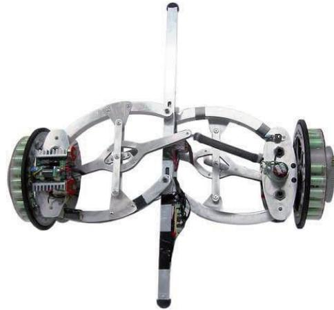
Fig. 17. “iHop v.3” prototype featuring independently actuated arms suspended via two spring-coupled linkages mirrored about the vertical axis.
