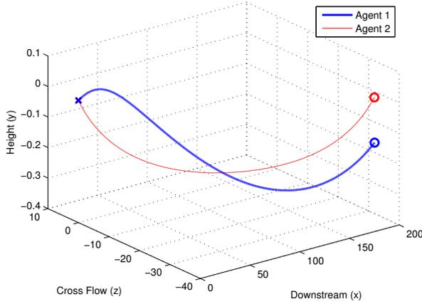
Fig. 4. Separation constants of  $C_z = 1$  and  $C_x = 5$ , direction anof a 2-agent system subject to idealized open channel flow.  $\times$  indicates starting location and  $\circ$  indicates final position. Initial positions at the origin with  $C_x = 0$ ,  $C_z = 1$ ,  $Q_q = 0$ ,  $Q_v = 0$ , and  $Q_T = 10I$
