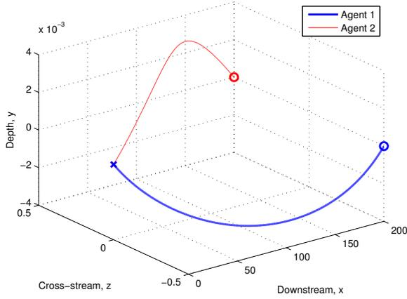
Fig. 3. Unit separation in the spanwise,  $z$ , direction of a 2-agent system subject to idealized open channel flow.  $\times$  indicates starting location and  $\circ$  indicates final position. Initial positions at the origin with  $C_x = 0$ ,  $C_z = 1$ ,  $Q_q = 0$ ,  $Q_v = 0$ , and  $Q_T = 10I$
