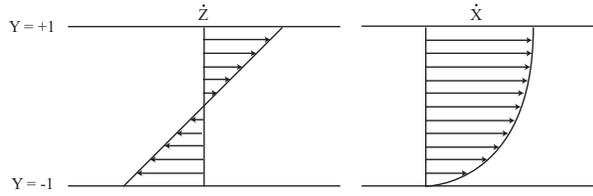
Fig. 2. Flow velocity profiles of an alternative flow configuration [cf. Fig. 1] resulting in the same simplified nonlinear model [compare (4) to (7)].
