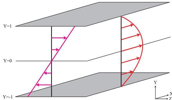
Fig. 1. Flow velocities of the basic flow considered in this paper, which is pressure-driven in the  $x$  direction and shear driven in the  $z$  direction.
