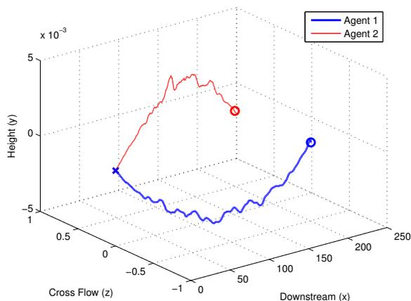
Fig. 7. Trajectory tracking for a scaled zero mean white noise excited background flow with ideal trajectories seeking unit separation in the spanwise,  $z$ , direction of a 2-agent system subject to idealized open channel flow.  $\times$  indicates starting location and  $\circ$  indicates final position. Initial positions at the origin with  $C_x = 0$ ,  $C_z = 1$ ,  $Q_q = 0$ ,  $Q_v = 0$ , and  $Q_T = 10I$
