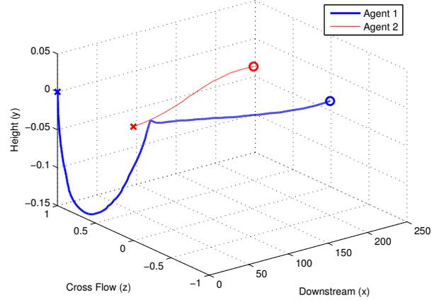
Fig. 5. Trajectory tracking for a perturbed initial state with ideal trajectories seeking unit separation in the spanwise,  $z$ , direction of a 2-agent system subject to idealized channel flow.  $\times$  indicates starting location and  $\circ$  indicates final position. Initial position  $\{x_1 = 0, y_1 = 0, z_1 = 1\}$  and  $\{x_2 = 0, y_2 = 0, z_2 = 0\}$  with  $C_x = 0$ ,  $C_z = 1$ ,  $Q_q = 0$ ,  $Q_v = 0$ , and  $Q_T = 10I$
