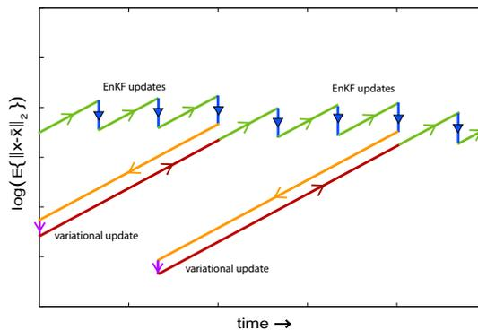
Figure 6. A cartoon illustrating the expected error for EnVE performed on a chaotic system. Exponential growth (linear growth in semi-log coordinates) in the expected error occurs during forward marches. Discrete reduction in the expected error occur at both the sequential updates and the variational update. Note that with a linear system, the variational update is necessarily zero, returning the estimate to its original value upon completion of the variational step.
