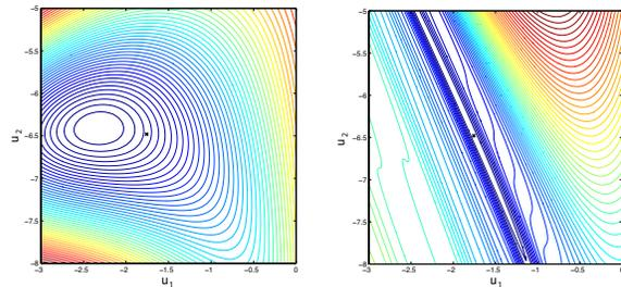
Figure 7. A cartoon illustrating the change in complexity of the optimization surfaces for a short variational window (left) and a long variational window (right). Also shown is the known truth model global minimum, which is more closely related to the global minimum of the highly irregular optimization surface of the longer window.
