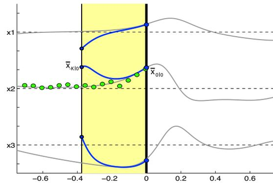
Figure 2. To determine the accuracy of the current estimate (that is, its correlation with the recent measurements), the ensemble at the current time is marched backwards using the system equations until the trajectory of the ensemble mean is significantly divergent from the observations. This gives the current best estimate at the past time,  $\bar{\mathbf{x}}_{-K|0}$ .
