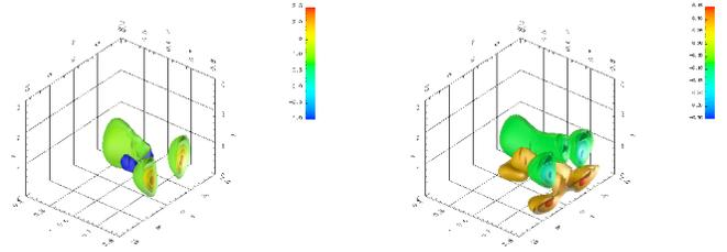
Fig. 3. Isosurfaces of  $K^0(x, y, z)$  relating (left) the streamwise component of the velocity  $u(x = 0.5, y, z)$ , and (right) the wall-normal component of the velocity  $v(x = 0.5, y, z)$  to the control input  $\phi(x, z = 0)$ . Control domain extension in  $x = [0.5, 0.8]$ . Minimization of the perturbation energy at  $x = 0.8$ .
