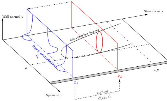
Fig. 2. Relation between the convolution control kernel and the control. The control  $\phi(x = x_k, z)$  is found by convolving the convolution kernel  $K^0$  in the plane  $x = x_k$  with the augmented state  $\mathbf{q}_0^a$  in the vicinity of the spanwise location  $z$ .
