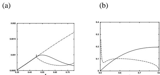
Fig. 4. (a) Evolution of the energy of perturbation  $E$  using (—) no control, (—) the present feedback control strategy, (- · -) the iterative adjoint-based control optimization strategy of [7]. (b) Evolution of the control energy using (—) the present strategy, (- · -) the adjoint-based strategy.
