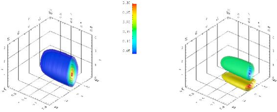
Fig. 1. Isosurfaces of  $K^0(x, y, z)$  (left) relating the streamwise component of the velocity  $u(x = 0.5, y, z)$ , and (right) relating the wall-normal component of the velocity  $v(x = 0.5, y, z)$  to the control input  $\phi(x, z = 0)$ . Note the control domain extension in  $x = [0.5, 0.8]$ .
