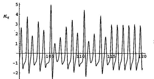
(d) Estimator designed with  $\alpha = 0.1$ ,  $\bar{x} = 0$ , and the nonlinear term dropped from the estimator equation (5). Lyapunov exponent  $\kappa_\infty = 0.01$ . The nonlinear term in the estimator is essential for good performance (cf. figure 2b).
