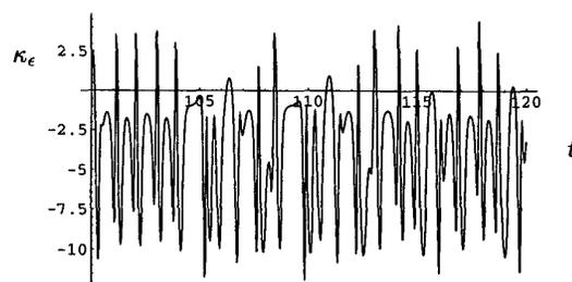
(b) Estimator designed with  $\alpha = 0.1$ ,  $\bar{x} = 0$ . The value of the Lyapunov exponent is  $\kappa_\infty = -3.95 < 0$ . This indicates that the state estimator is stable more than it is unstable, and thus the state estimate will converge to the uncontrolled state when  $x_e$  is small. Note that estimator convergence is attained even though the estimator error does not decrease uniformly over the entire path of the attractor.
