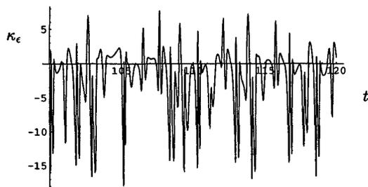
(c) Estimator designed with  $\alpha = 0.1$ ,  $\bar{x} = \bar{x}$ . Lyapunov exponent  $\kappa_\infty = -2.33 < 0$ . It is found that linear estimator feedback designed with  $\bar{x} = 0$  has better convergence properties (cf. figure 2b).
