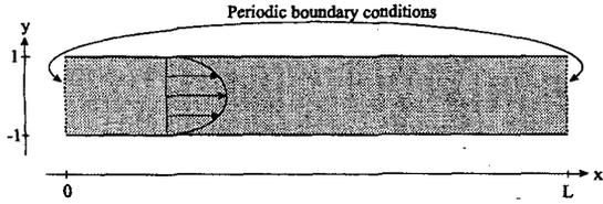
Figure 1: Geometry of the flow problem.
