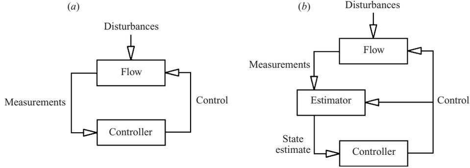
FIGURE 2. Examples of practical feedback control configurations based on limited noisy flow measurements. The unknown feedback coefficients in both configurations may be optimized numerically with the techniques based on the optimization approach developed in this paper. (a) Output feedback configuration, (b) estimator-based configuration.
