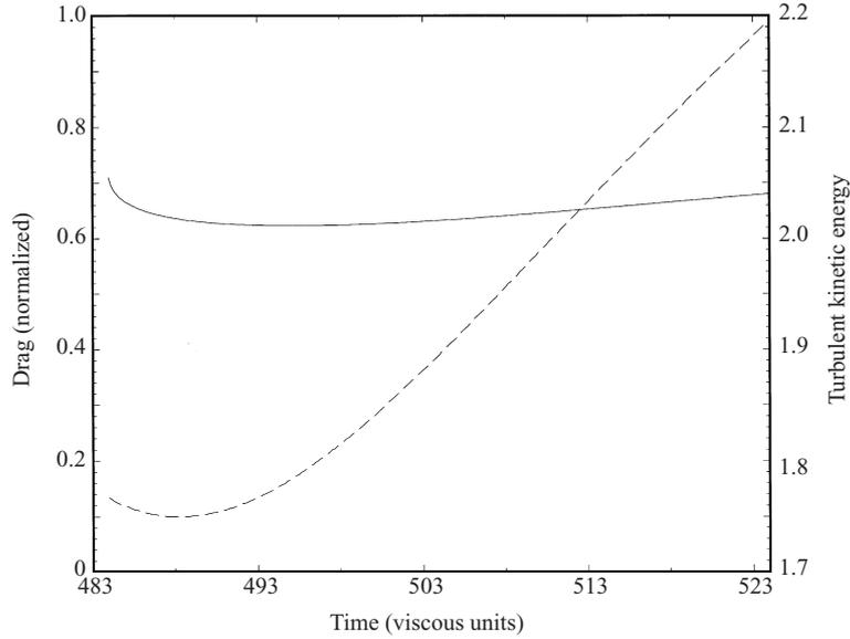
FIGURE 14. Response of system on  $[t, t + T]$  in a controlled simulation ( $\mathcal{J}_{\text{TKE(ter)}}$  formulation,  $T^+ = 40$ , and  $Re_\tau = 180$ ) with control turned off at  $t^+ = 483$ : —, drag (scale at left); ---, TKE (scale at right). The faster rise of the TKE indicates that it is a more sensitive indicator of turbulence regeneration in the flow.
