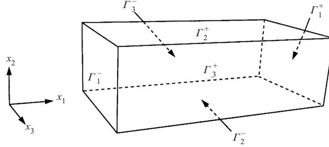
FIGURE 3. Channel flow geometry. The interior of the domain is denoted  $\Omega$  and the boundaries of the domain in the  $x_i$ -direction are denoted  $\Gamma_i^\pm$ . Unsteady wall-normal velocity boundary conditions are applied on the walls  $\Gamma_2^\pm$  as the control, with periodic boundary conditions applied in the streamwise direction  $x_1$  and spanwise direction  $x_3$ .
