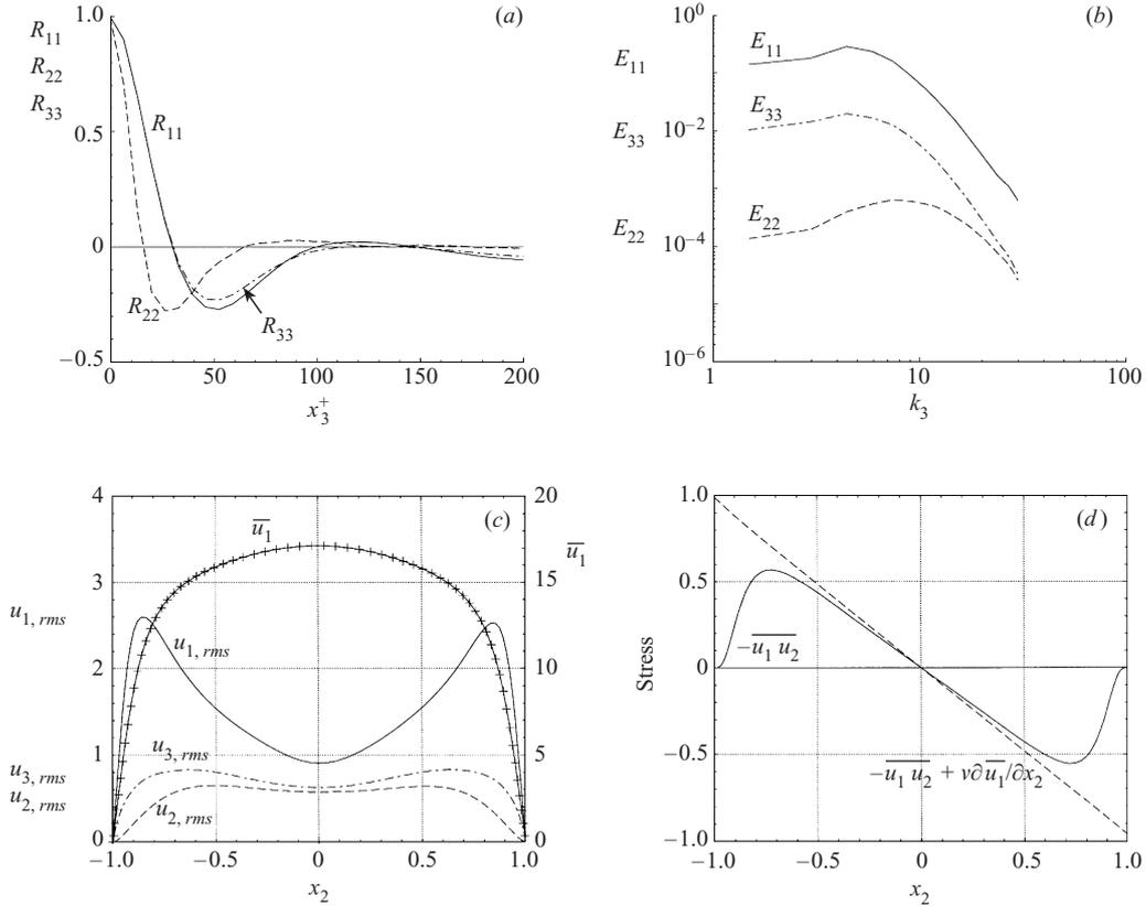
FIGURE 5. Selected time-averaged statistics of the uncontrolled turbulent channel flow at  $Re_\tau = 100$ : (a) spanwise two-point correlations at  $x_2^+ = 5.4$ ; (b) spanwise one-dimensional energy spectra at  $x_2^+ = 5.4$ ; (c) profiles of r.m.s. velocity fluctuations (left-hand scale) and mean velocity (right-hand scale); (d) profiles of Reynolds stress (—) and total stress (-----).
