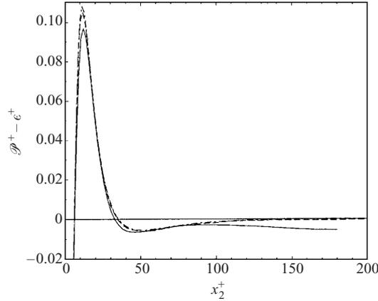
FIGURE 8. Excess energy production,  $\mathcal{P} - \epsilon$ , in wall units, as a function of distance from the wall. Data compiled by Jimenez (1999), for uncontrolled turbulent channel flows at: —,  $Re_\tau = 180$ ; ----,  $Re_\tau = 395$ ; -·-,  $Re_\tau = 590$ ; see Jimenez (1999) for descriptions of the various different computations reported in this figure.
